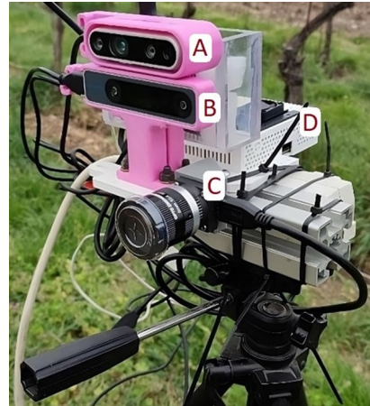
Fig. 1: Image of the proposed acquisition set-up. (A) depth camera D435i, (B) tracking camera T265, (C) Basler RGB camera with optics, (D) Nvidia Jetson Nano.
