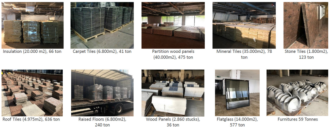
FIGURE 4: Overview of the stocks of reclaimed building components disassembled from the World Trade Centre towers and destined to onsite/offsite reuse.
