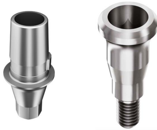
Figure 9. Ti-Base titanium Grade V (left) used for one-piece restoration directly connected to the fixture. GFA (right) screwed to the implants and used for two-pieces restoration connected to the GFA.
