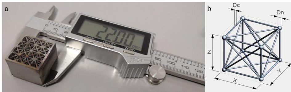
Fig. 1. (a) square-based lattice sample with solid shell; (b) design of Face Centered Cubic (FCC) unit cell.
