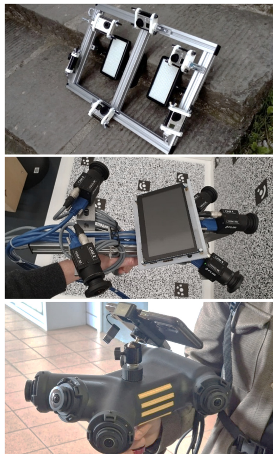
Figure 5. Milestones in the development of Ant3D. Multi-camera GoPro rig from 2018 FINE Benchmark (top), Ant3D v1 (centre), and first industrialized prototype Atom-Ant3D (bottom).
