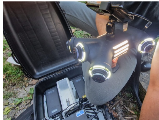
Figure 1. Latest version of the Ant3D multi-camera system. The picture shows the first production prototype developed by Gexcel srl with the control backpack.
