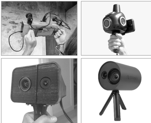
Figure 2. Examples of recent multi-camera portable visual SLAM systems from research: Gupho (top left, Torresani et al., 2021); Looq qCam (top right, Looq AI); system from Ortiz-Coder and Sánchez-Ríos, 2019 (bottom left); Stonex XVS vSLAM scanner (bottom right).
