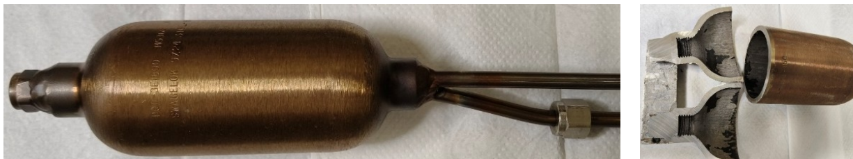
Figure 6.8. The 316L vessel after \text{GeCl}_4 thermal stress for 100h at 450°C
