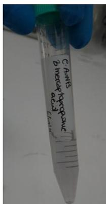
**Figure 3.8:** Gold nanoparticles functionalized with 3-mercaptopropionic acid dissolved after resuspension.
