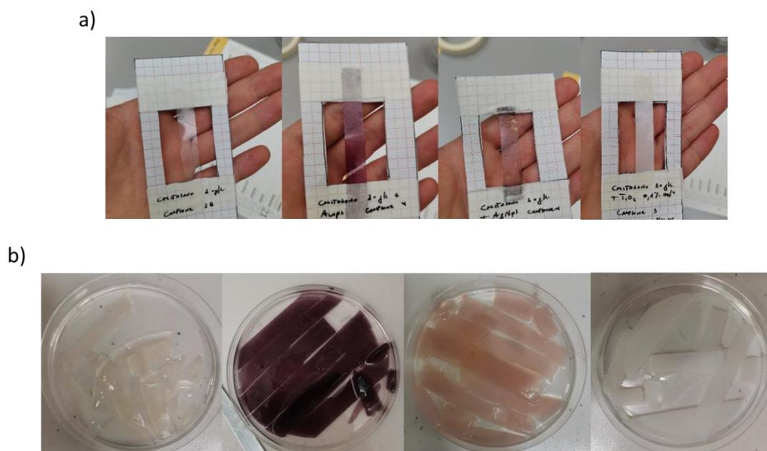
**Figure 4.18:** a) paper frames prepared for the strips 40mm x 10 mm obtained from dry films. b) 40mm x 10 mm strips cut from wet films.
