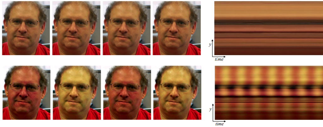
Figure 3: Eulerian Video Magnification method to detect the human heartbeat. Top: Four frames from the initial video recording, and a vertical scan line of the input plotted over time. Bottom: the same four screenshots with the subject's heartbeat signal intensified, and a vertical intensified scan line of the input plotted over time. In the input sequence the signal is unnoticeable, but in the magnified sequence the fluctuation is obvious. [4]
