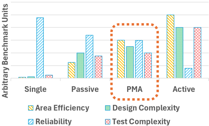
Figure 3.9: Comparison of Area Efficiency, Design Complexity, Reliability, and Test Complexity for different test infrastructure architectures: Single Padded, Passive Arrays, Passive Matching Arrays, and Active Arrays
