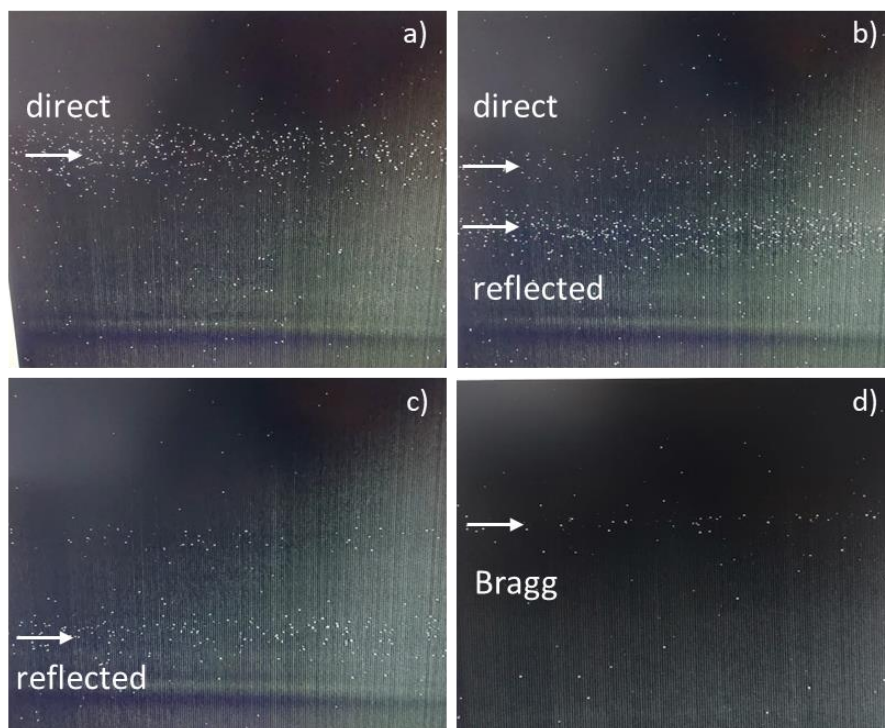
Figure 36 – Alignment procedure seen from the CCD camera. First only the direct beam is visible (a). Then, the direct beam splits and also the reflected beam is visible (b), becoming more and more intense (c). By further tilting the multilayer the Bragg angle is found (d).
