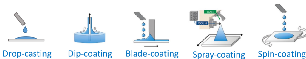
Figure 2.4. Thin film deposition techniques of hybrid or inorganic perovskite from precursor salts dissolved in solution.
