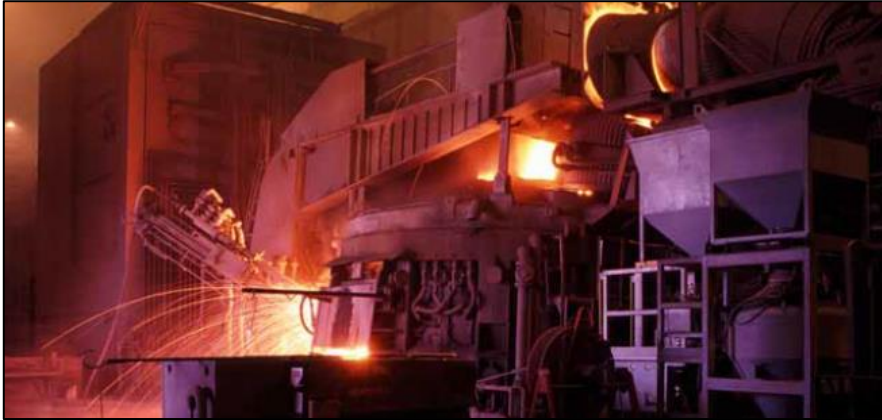
Figure 2-3: Electric Arc Furnace (EAF) [2].
