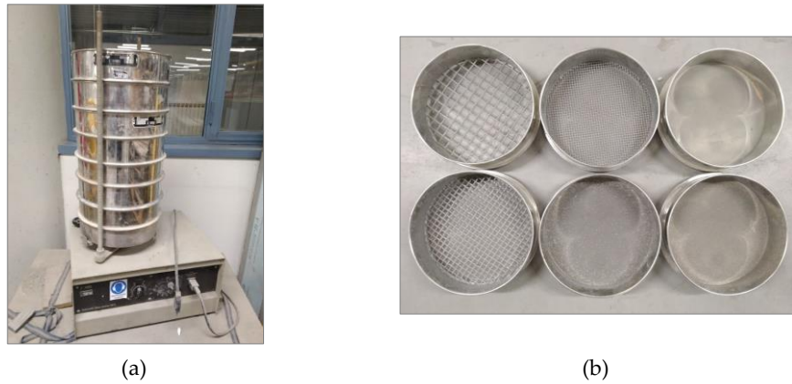
Figure 5-6: Vibrating screen (a) and some of the sieves (b) used for the granulometric analysis. Photos taken by Alan Piemonti.
