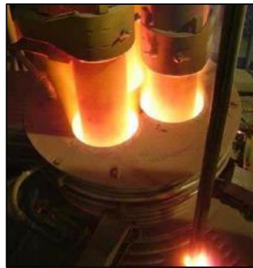
Figure 2-4: Ladle Furnace (LF) [1].
