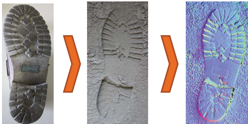
Fig. 12 Comparison of shoe, photograph and 3D data of impression in sand under laboratory conditions
