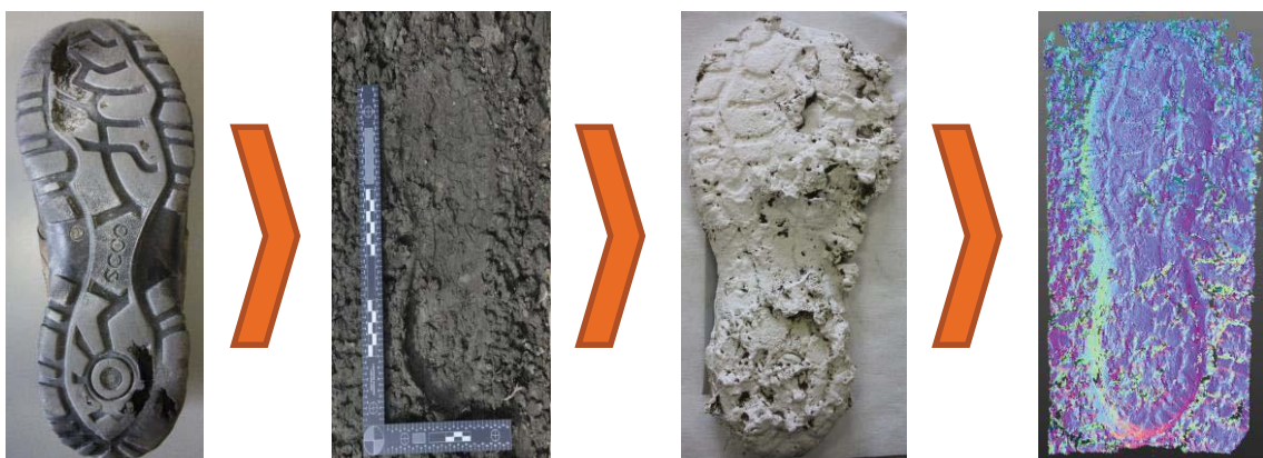
Fig. 13 Comparison of shoe, photograph, plaster cast and 3D data of impression in clay under field conditions
