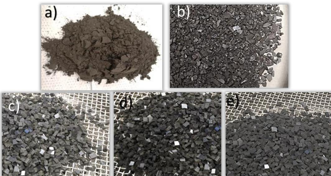
Figure 81 Samples subjected to the leaching test. a) free EAF slag (grain size lower than 100 $\mu$ m); b) free EAF slag (grain size lower than 4mm); c) NBR filled 100%slag cut in particle size of less than 4 mm; d) NBR filled 50%slag cut in particle size of less than 4 mm; e) standard NBR cut in particle size of less than 4 mm.
