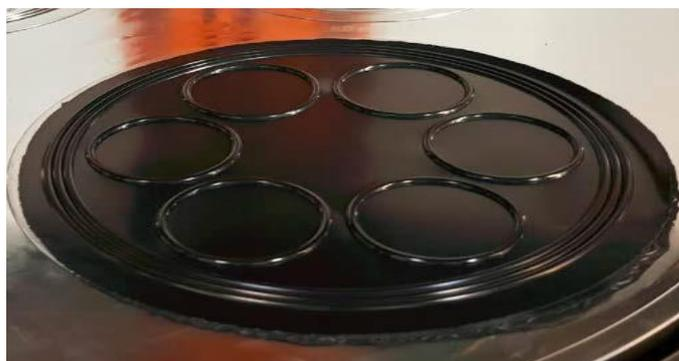
Figure 10 Example of compression moulded parts with thin film of burr to be removed.
