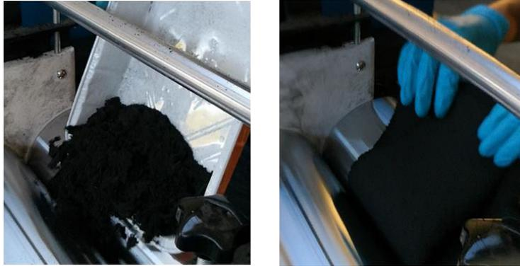
Figure 107 During the calendaring process ELT powder (beginning of the process) is transformed into a compound (end of the process).
