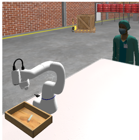
Figure 5.12: Placing the test tube in the divider
