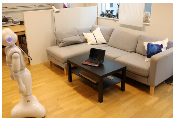
Figure 7.2: Pepper taking images of a laptop and asking a human to manipulate it for learning the property Folded .
