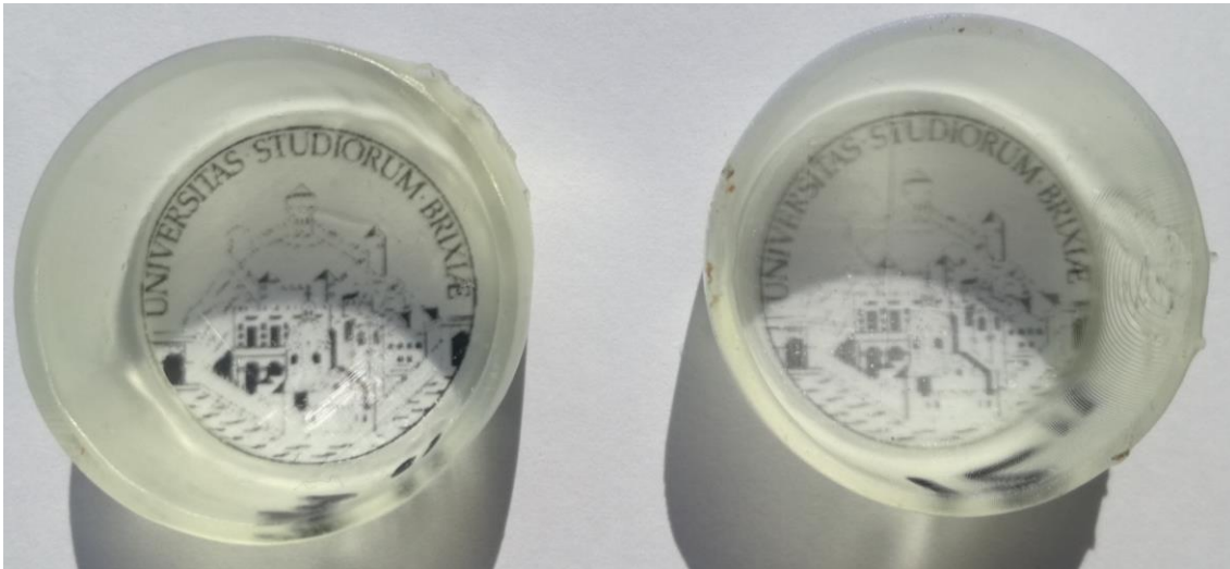
Figure 4: Comparison between test n.3 that passed the transparency test (left) and test n.12 that did not (right).
