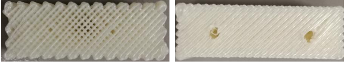
Fig. 8 Drilling holes on the samples with a density of 25% (left) and 87.% (right).
