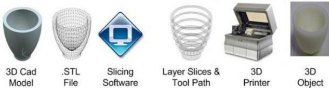
Fig. 1 Additive manufacturing steps [6].
