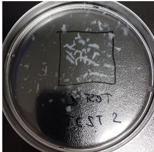
Fig. 1 0.5% dECM structure shattered after the washing of the supporting bath.
