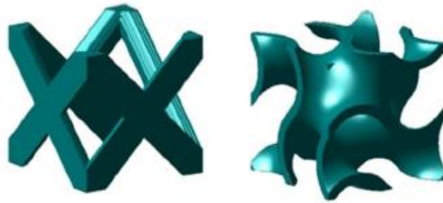
Fig. 6 Example of strut-based (left) and triply periodic minimal surface (right) structures [42].
