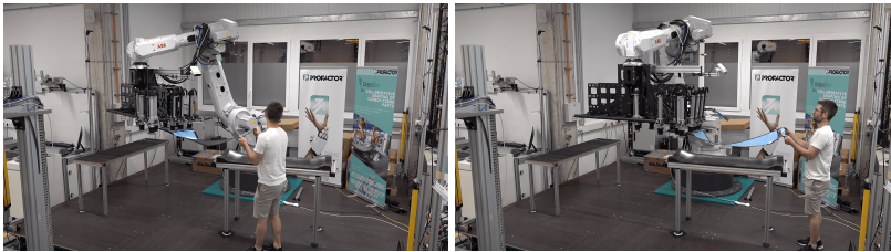
(e) The human and the robot transport the ply towards the goal pose - collaborative transport with role arbitration (f) The human leads the task toward the goal pose - smooth leader role switch from human to robot
