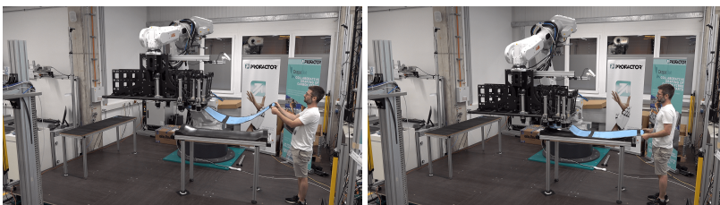
(g) The robot leads the task precisely to the goal pose - robot leader (h) The robot approaches the mold to allow precise draping
