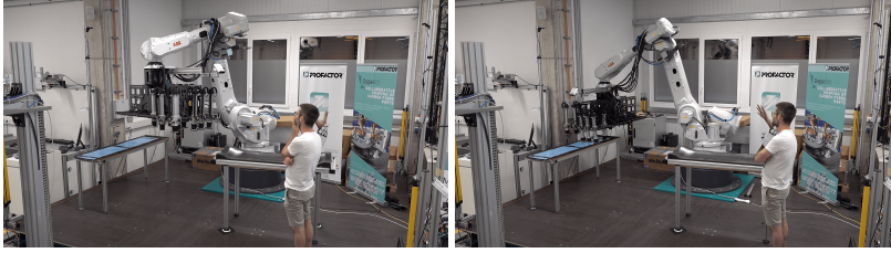
(a) The robot approaches the ply - autonomous motion (b) The robot grasps the ply - autonomous motion
