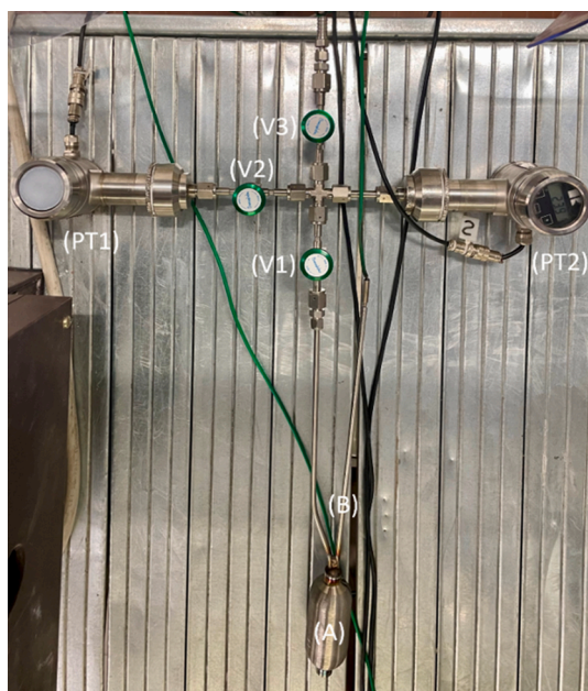
Fig. 4. Main components of the thermal stability test: the AISI 316L cylinder (A), the housing of the temperature probe (B), the low-pressure scale pressure transducer (PT1), the high-pressure scale pressure transducer (PT2), the main valve isolating the cylinder (V1), the valve protecting the PT1 from overpressure (V2), the valve connecting the circuit to the environment (V3). Figure adapted from authors previous work [41].
