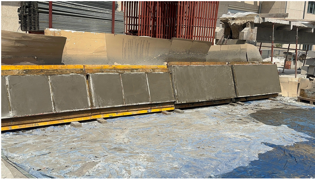
Figure 4.7: Sprayed panels prepared for the EN 14488-3 Method B 3PBT notched panel test [16], along with the large panels intended for sawn-cut beams for the EN 14651 3PBT notched beam test [7].
