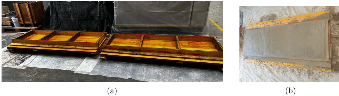
Figure 4.8: Panel casting procedure for the EN 14488-3 Method B [16] test methodology: (a) Moulds used for casting the panels; (b) Cast panel specimen.
