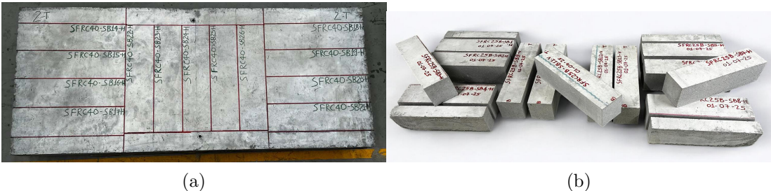
Figure 4.12: Saw-cut layout and resulting beams for the EN 14651 [7] 3PBT: (a) Saw-cut layout of the large sprayed panel; (b) Saw-cut beam specimens.
