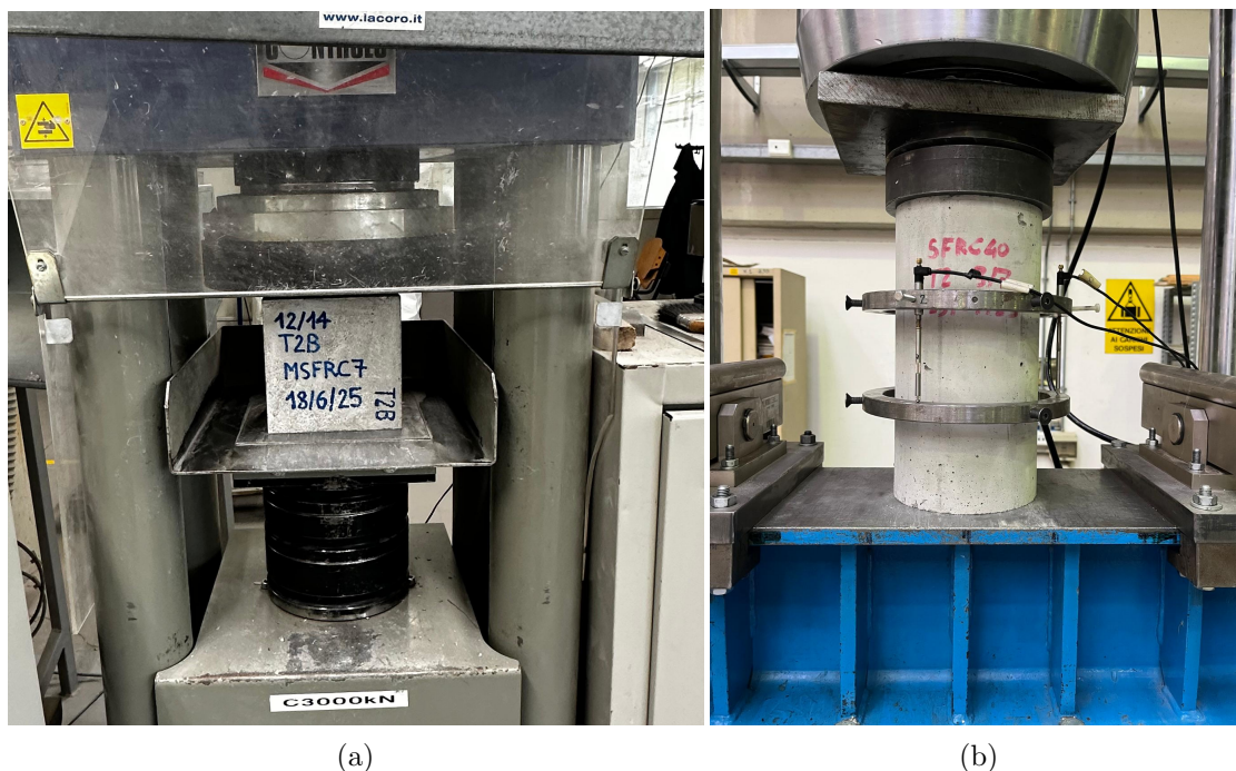
Figure 4.27: Experimental setup: (a) Compressive strength test using a 3000 kN hydraulic press; (b) Elastic modulus test with displacement transducers.
