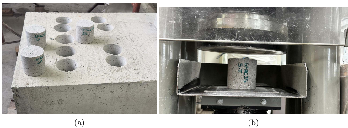
Figure 4.11: Compressive strength testing of cored cylinders extracted from sprayed panels: (a) Cored cylinders obtained from the sprayed panels ; (b) Compressive strength test set-up for the cored cylinders.
