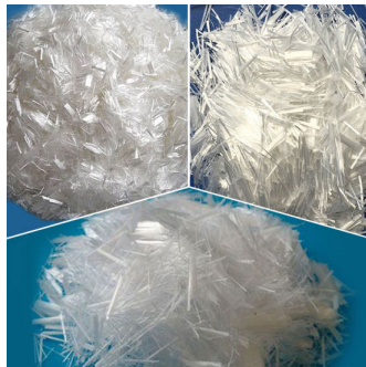
Figure 2.31: Micro-synthetic fibres (images sourced from manufacturer's data sheets).
