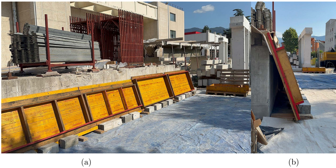
Figure 4.4: Outdoor panel layout prior to spraying: (a) Overall 20°-inclined layout of panels; (b) Detail view showing the 20° inclination of the plywood formwork.
