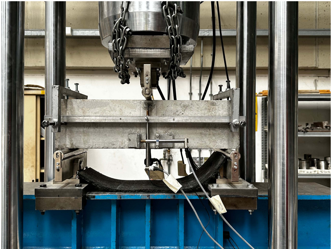
Figure 4.20: Set-up for EN 14651 [7] with INSTRON 1274 closed-loop servo-hydraulic testing machine.
