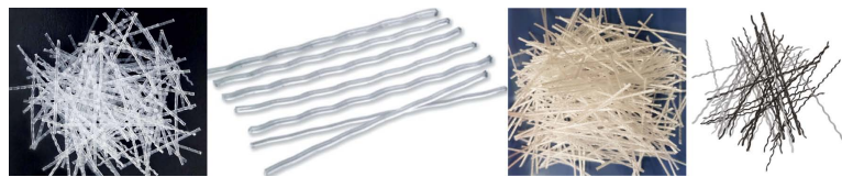
Figure 2.30: Various types of macro-synthetic fibres (images sourced from manufacturer's data sheets).
