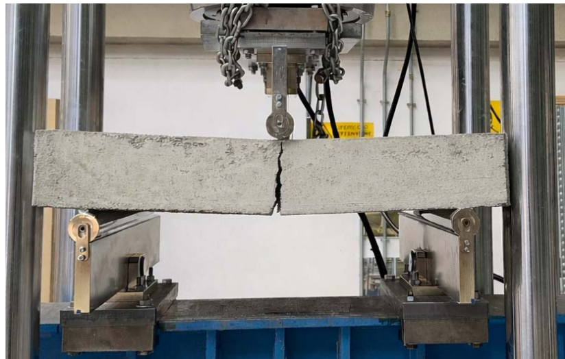
Figure 4.19: EN 14488-3 Method B notched sprayed panel after testing, showing crack formation and panel deformation [16].
