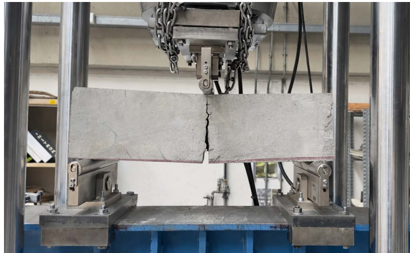
Figure 4.23: EN 14651 saw-cut notched beam specimen after testing, showing crack formation and beam deformation.
