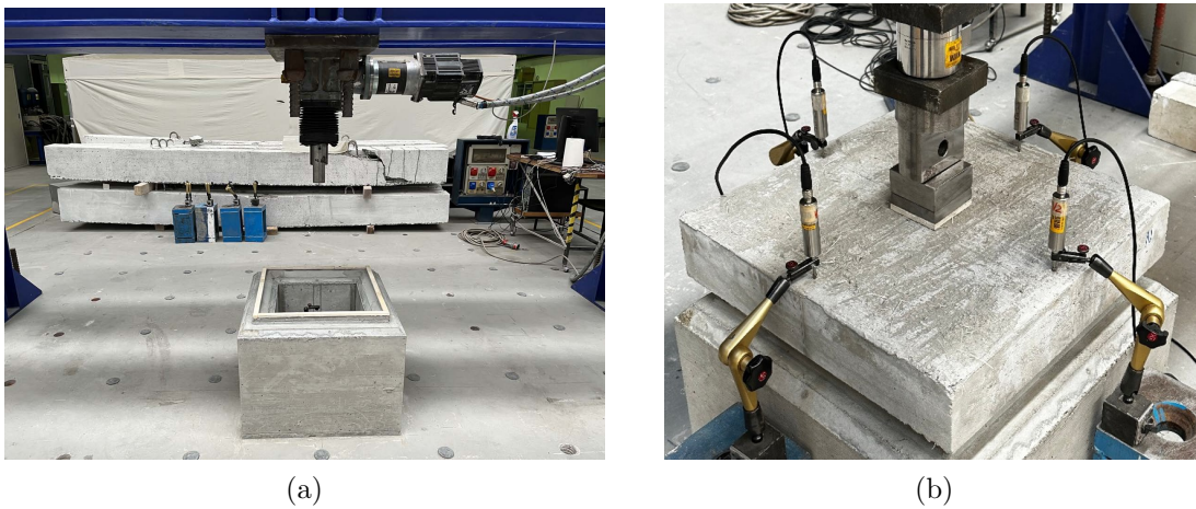
Figure 4.24: Energy absorption test according to EN 14488-5 :(a) Electromechanical screw jack and rigid foundation support set-up; (b) Detail test setup.
