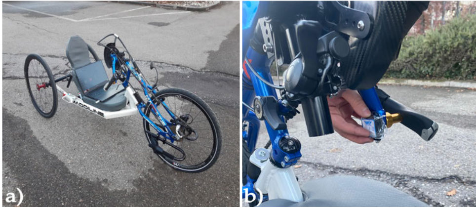
Fig. 4.2: a) The Race-X handbike employed in the experimental tests; b) IMU sensor mounted on the handbike handlebar. Reproduced from [16] with permission from Springer Nature.
