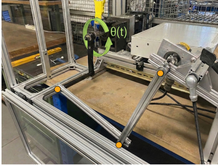
Fig. 3.1: The green circular arrow, denoted as \theta(t) , indicates the time-dependent rotational angle applied by the motor to the crank. The orange circular markers signify the location of the revolute joints representing shoulder, elbow, and wrist connecting arm and forearm.
