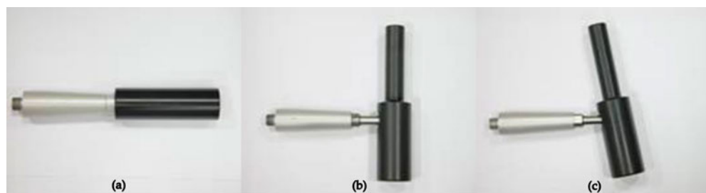
Figure 16. Handle angle configurations analyzed by Abel et al. [21]: from the left, (a) horizontal (0°), (b) vertical (90°), and (c) diagonal (10°) configuration. Source: Abel et al., 2015 [21].
