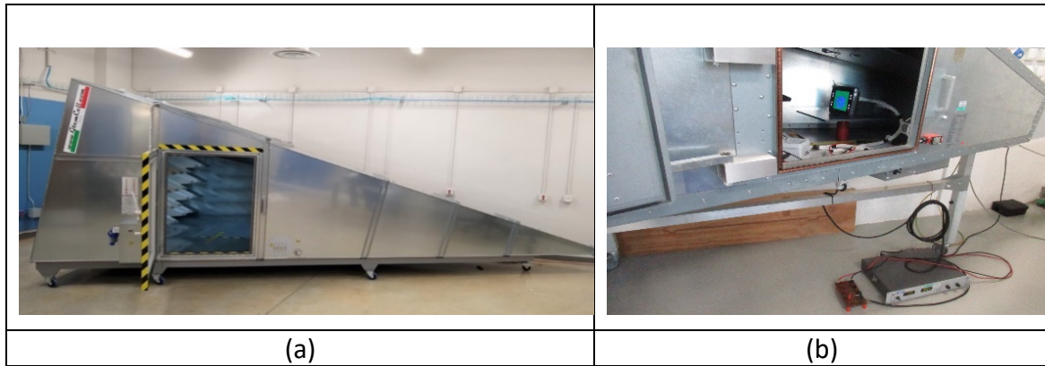
Figure 26. GTEM cell setup for EMC testing: (a) external view of the GTEM chamber, (b) dashboard unit positioned inside the test section with RF instrumentation.
