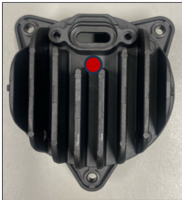
Figure 23. Position of the thermocouple on the rear housing used for temperature-step (derating) test.
