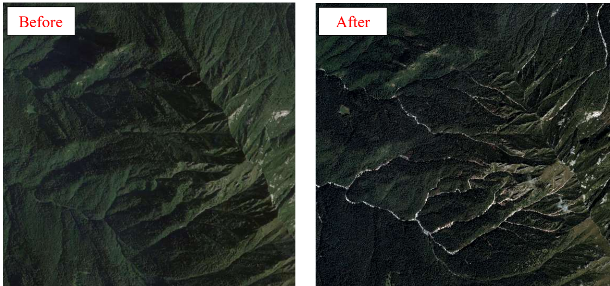
Figure 2.19 A comparative view of the change in morphology of the catchments of Re (south) and Cobello (North), aerial view taken from Google Earth before the event and immediately afterwards. There are more than 40 unstable source areas that contributed to the debris flow that damaged the town of Niardo.
