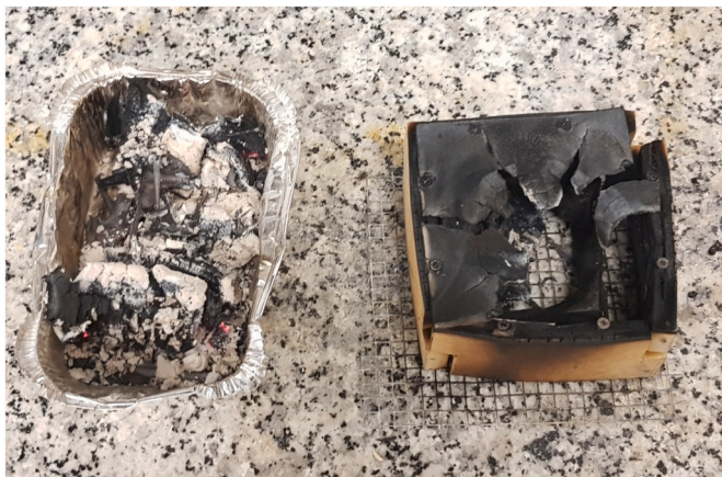
Fig. 17. Sample condition after the fire performance test for the polyamide on metal grid case.
