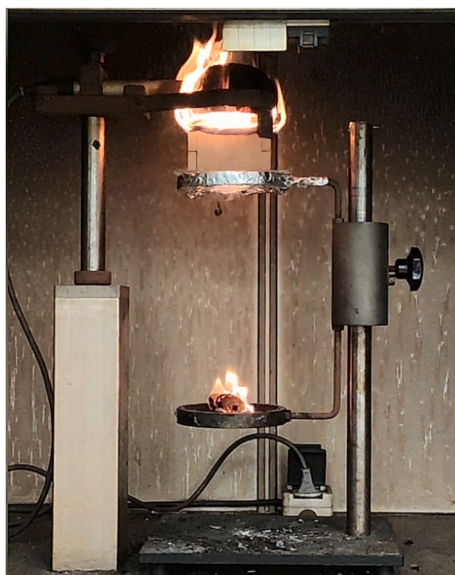
Fig. 18. Dripping of ignited material for the polyamide on a metal drip case.
