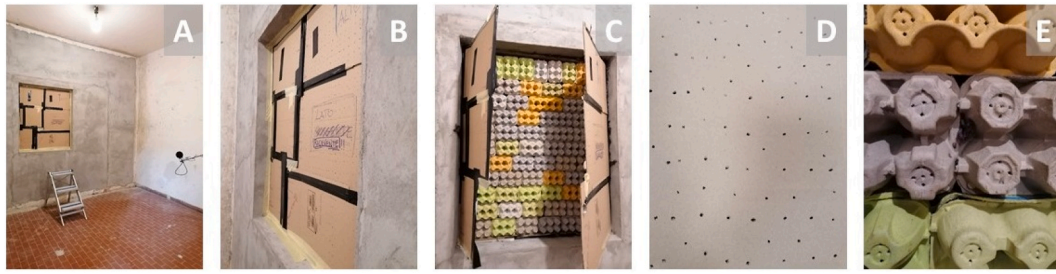
Fig. 11. Detailed view of the constructed panel and its setup at CNR sound transmission room. (A) Specimen installed in the sound transmission room. (B) Panel external surface. (C) Insulating core. (D) Example of the holes drilled on the external case. (E) Drilled egg carton domes.
