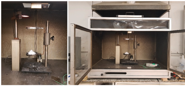
Fig. 14. Dripping test device.
