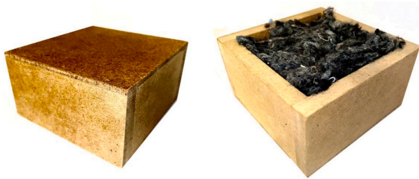
Fig. 15. Cladding sample used in the fire performance tests.
