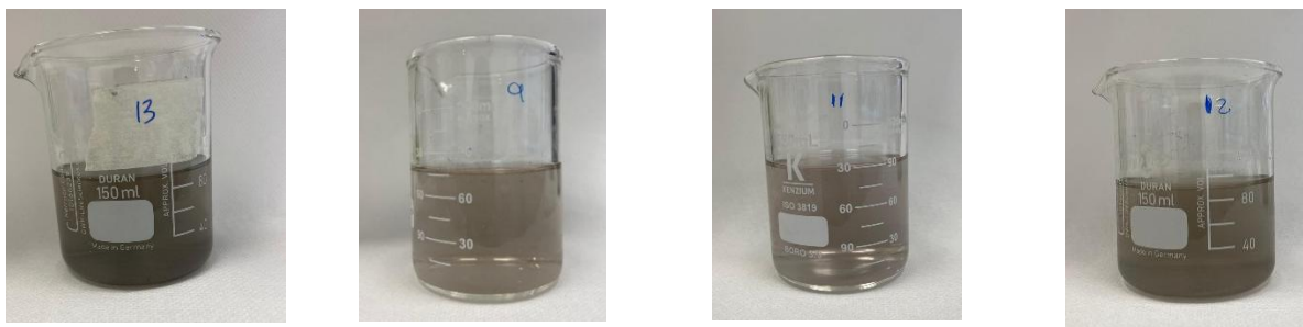
Figure 4.18. Visual comparison of wastewater samples treated under different flocculation conditions with chitosan and C-PAM. From left to right: exp. 1, exp. 2, exp. 3, exp. 4. The images highlight the effect of C-PAM addition in promoting the aggregation of microflocs into larger and more compact structures, resulting in improved sedimentation and clearer supernatant compared to treatments with chitosan alone.
