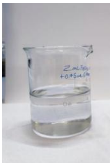
Figure 4.23. Wastewater sample after the treatment with \text{FeCl}_3 and filtration stage
