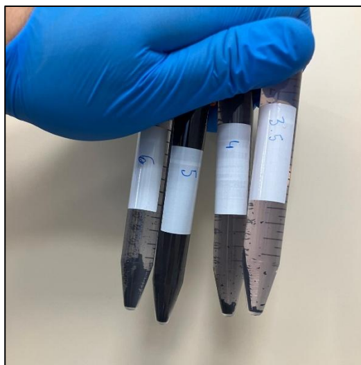
Figure 4.2. Visual appearance of samples after acidification, filtration, and centrifugation, highlighting floc formation and phase separation.
