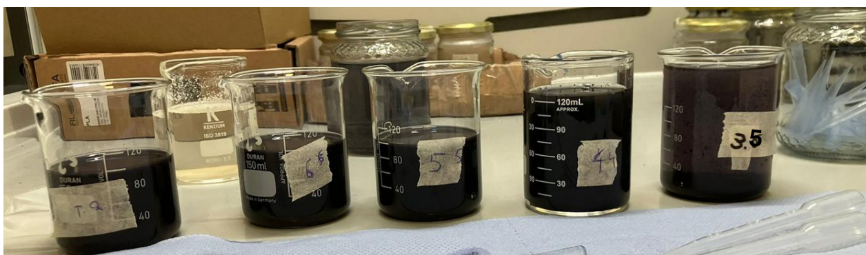
Figure 4.1. Experiment for the identification of the optimal pH. From left to right: raw sample, pH 6 sample, pH 5 sample, pH 4 sample, and pH 3.5 sample.
