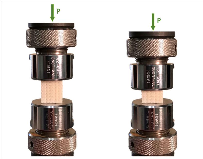
Figure 3.6: Compression tests on 3D-printed cellular structures.
