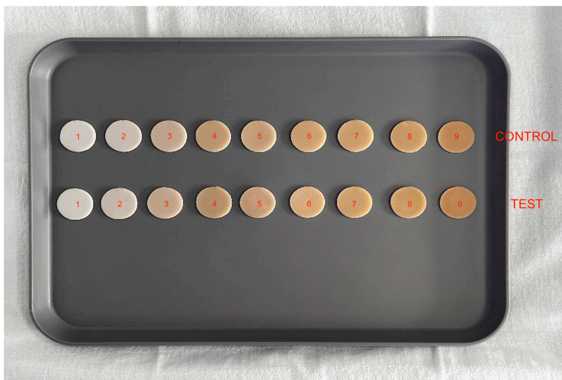
Figure 1. Nine control discs and nine test discs arranged following the Micerium chromatic scale (1-2-3-4-5-6-7-8-9) (incremental order).
