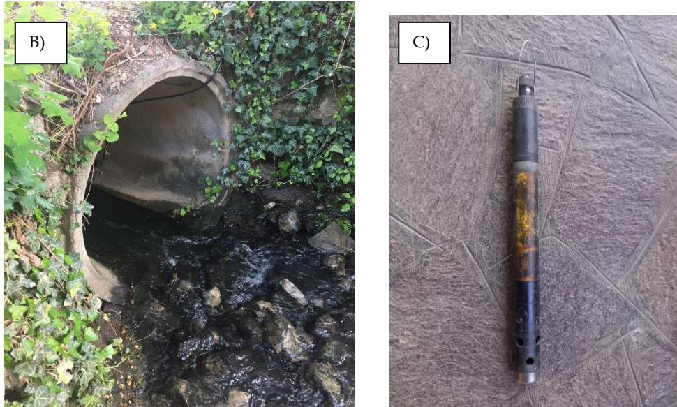
Figure 3.35 A) Watershed of Rì and location of the station B) location of IS1 where the water level probe is installed (a black wire is visible entering the pipe) C) YSI probe for specific conductivity
