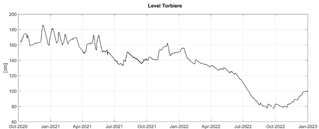
Figure 3.4 Daily-averaged water levels at Torbiere monitoring station – series of Hobo and Mobrey measurements from October 2020 to January 2023
