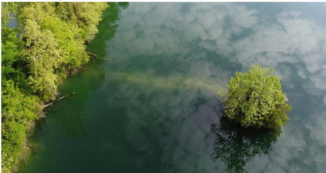
Figure 3.31 Drone picture of the submerged sill between the Southern pond (low portion of the picture) and the Northern pond (top portion of the picture). Credits: UniBS hydraulic group 29/04/2022)
