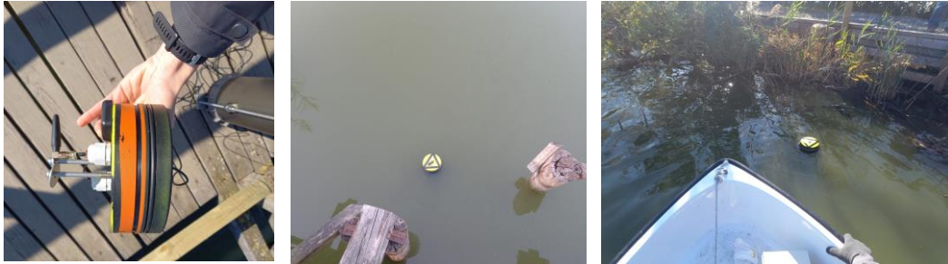
Figure 5.7 a) the cap of the casing, b) the drifter seen from above, right after the deployment from one of the piers, c) the recovery 1 day after, after reaching the drifter with a boat.
