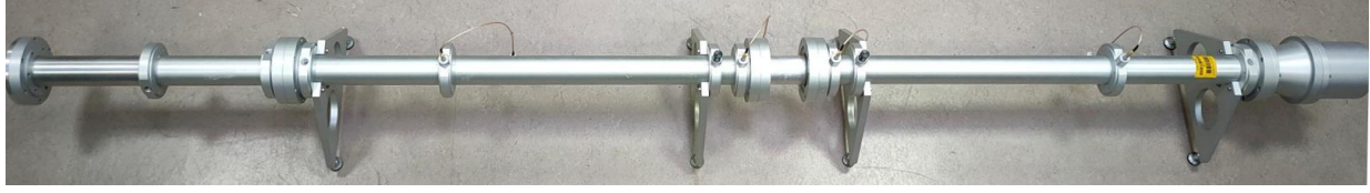
Fig. 5 Picture of the impedance tube including the anechoic termination (left), the sample holder (centre), and the loudspeaker (right).
