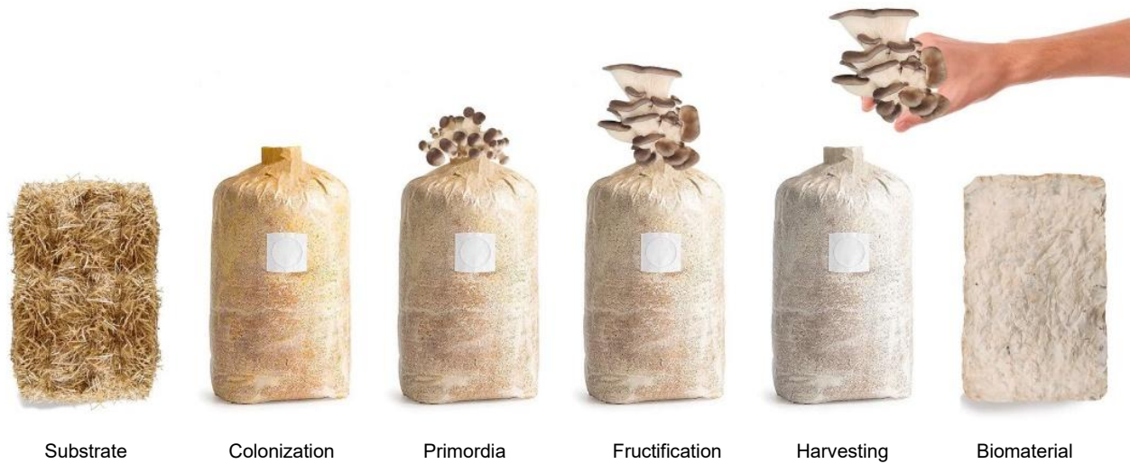
Fig. 1 Mush2Biom production process from edible mushroom cultivation to mycelium-based composites
