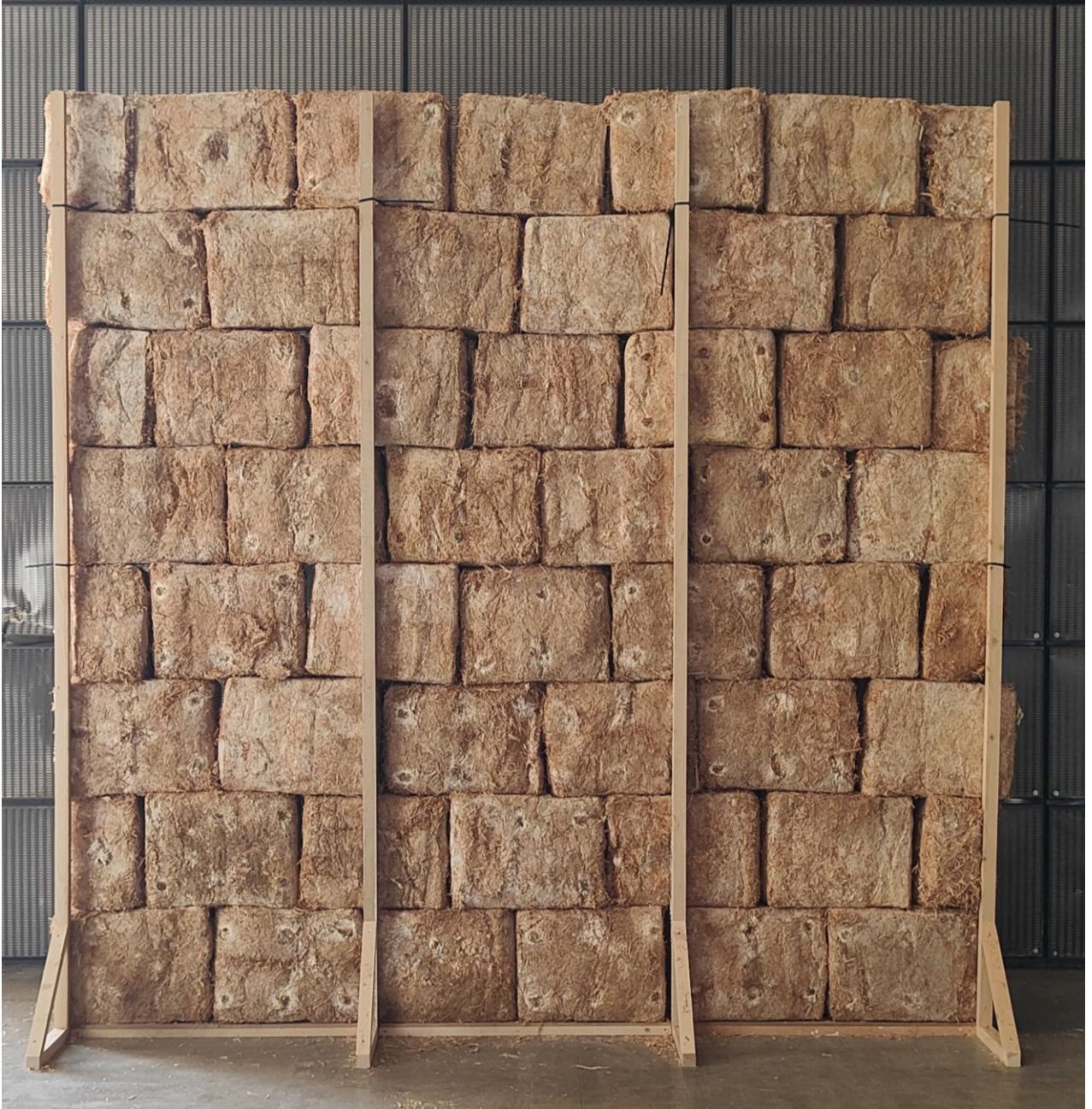
Fig. 3 Mush2bioM full-scale prototype wall (3 × 3 m) constructed using dehydrated SMS-based MBCs. The modular assembly demonstrates the material's ability to form self-supporting vertical structures without additional chemical treatments or compaction. The system highlights the potential of MBCs for temporary, low-impact architectural applications such as fairs trade, exhibition walls and pavilions.
