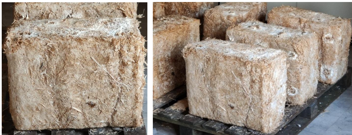
Fig 1 SMS-based MBC specimens used for compression testing (sample 1-5). Samples were used as cultivation substrate for edible mushroom production and then transformed into MBCs measuring 500×350×250 mm.
