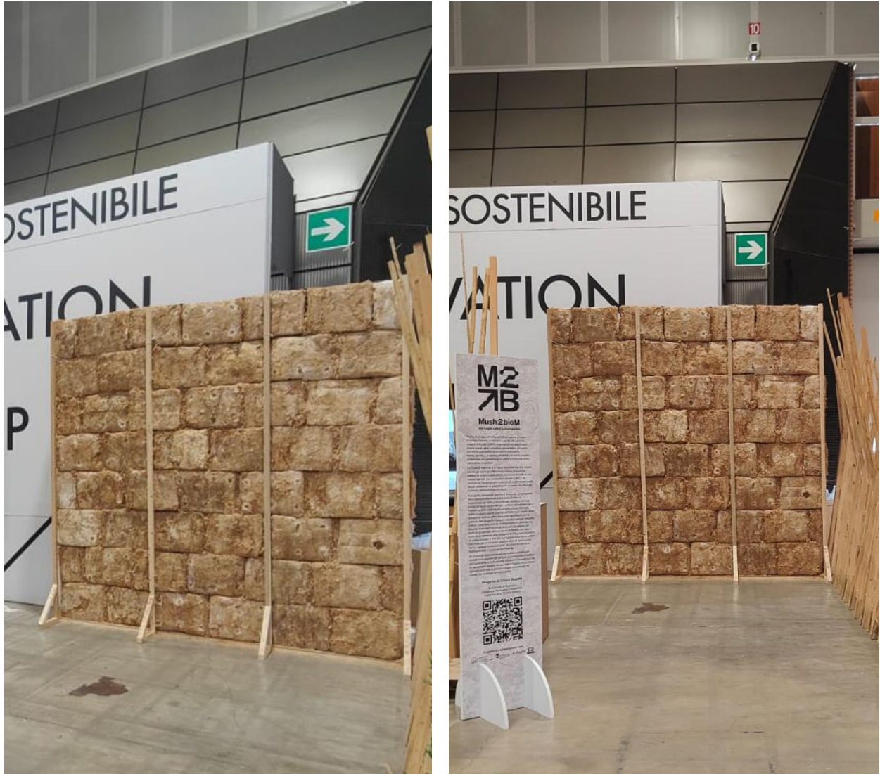
Fig. 4 This Mush2Biom full-scale prototype wall (3 × 3 m) was built and exhibited at FUTURA EXPO, Italy, using dehydrated SMS-based MBC panels. The modular system demonstrates the material's capacity to form self-supporting vertical structures without chemical treatments or mechanical compaction. The prototype showcases the potential of these biomaterials for temporary, low-impact architectural applications such as trade-fair installations, exhibition walls, and lightweight pavilions.
