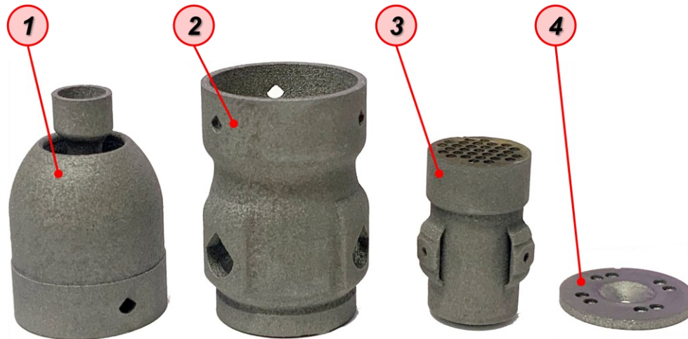
Figure 4.45 LPBF-manufactured Ta FEBIAD ion source components presented in paragraph 4.7.1 . (1) Cathode, (2) discharge chamber, (3) anode, (4) extraction system.
