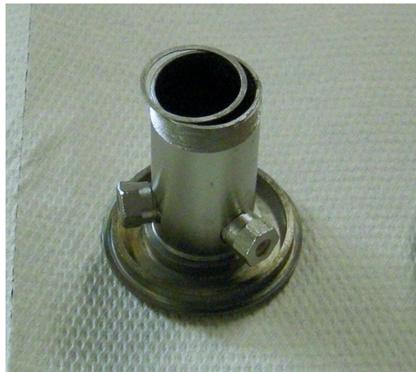
Figure 7.10: Discharge chamber assembled with the extraction flange
