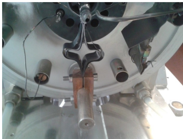
Figure 7.21: Anode wire and electrical connection attached to the chamber
