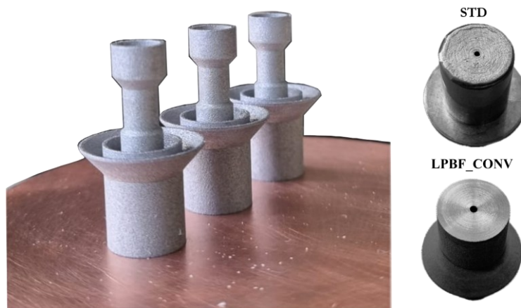
Figure 4.16 LPBF_conv cathodes produced at DIAM lab of INFN-Padova section.
