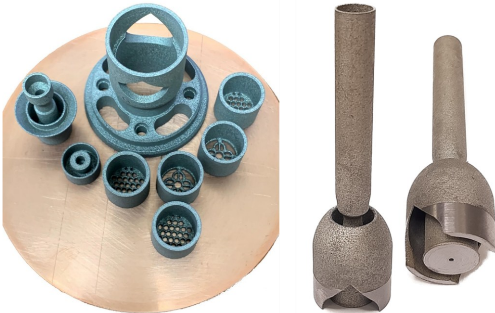
Figure 6.14 Thermionic emission setup parts and cathodes produced via LPBF process.
