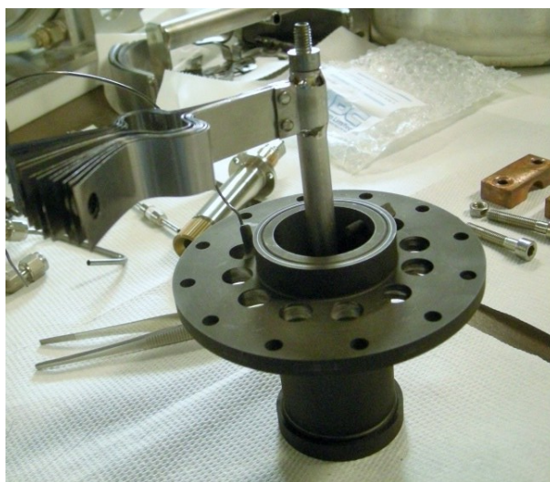
Figure 7.18: Assembling of the transfer line
