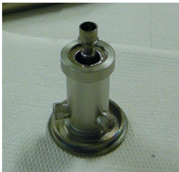
Figure 7.12: Anode - Cathode sub assembly
