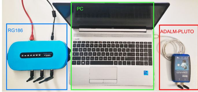
Figure 4.2: The experimental setup including the LoRaWAN GW from Laird, the SDR, and the PC.
