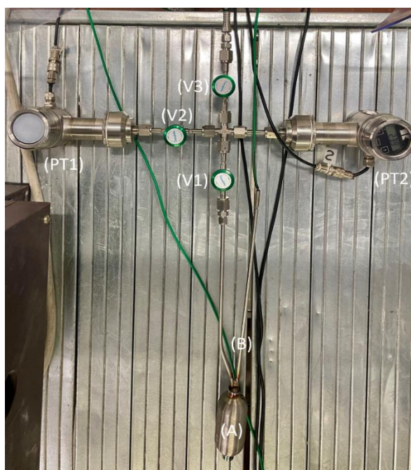
Figure 4. Main components of the thermal stability test: the AISI 316L cylinder (A), the housing of the temperature probe (B), the low-pressure scale pressure transducer (PT1), the high-pressure scale pressure transducer (PT2), the main valve isolating the cylinder (V1), the valve protecting the PT1 from overpressure (V2), the valve connecting the circuit to the environment (V3). Figure adapted from authors previous work [41].
