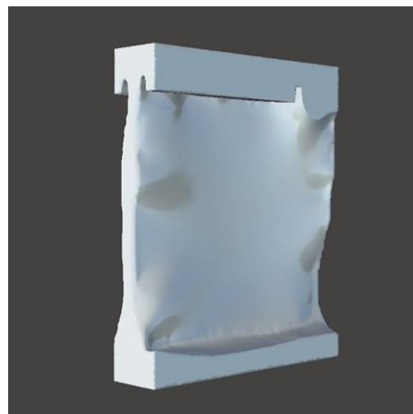
Fig. 2.11 Nasal septum module. The square-section parts on the top and on the bottom were made with Plane Cut function to facilitate the fabrication of the module and its insertion in the frame.
