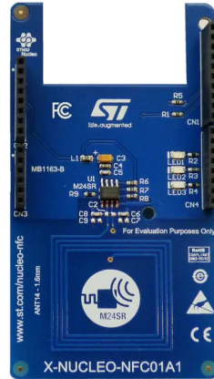
Figure 2.14: X-NUCLEO-NFC01A1 board: Top view, highlighting compatibility with STM32 and Arduino UNO R3 MCUs
