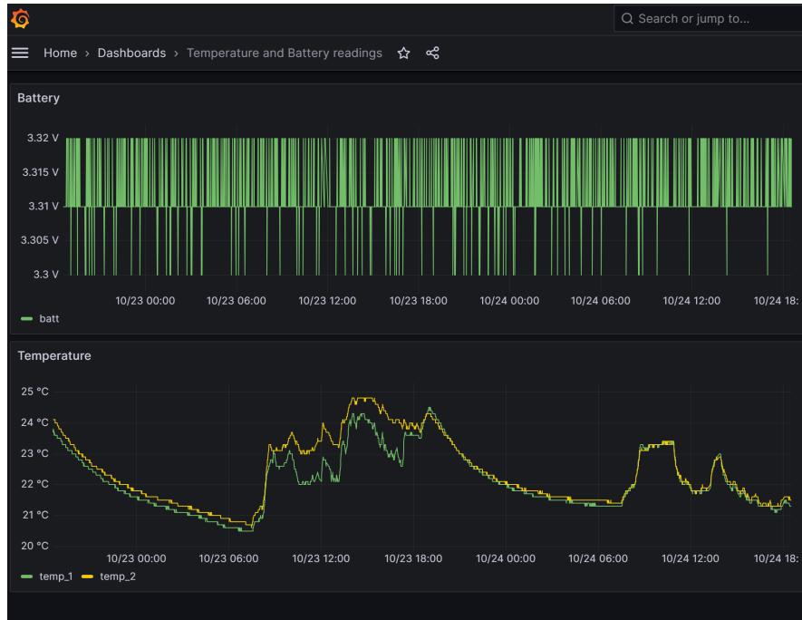
Figure 4.9: Grafana dashboard showing battery and temperature sensor readings
