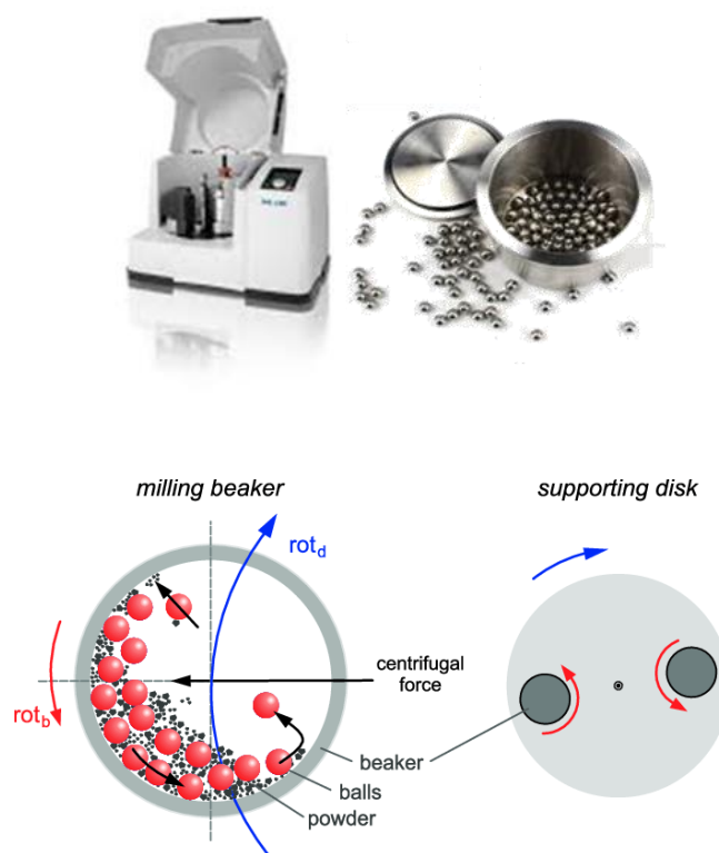
Figure 1.1 Planetary ball-mill apparatus and illustration of the planetary movement of grinding jars 27
