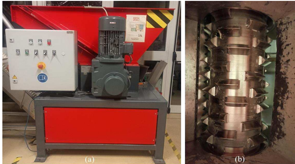
Figure 3.7: Single shaft shredder (a) and shredding chamber with single shaft and fixed blade (b)
