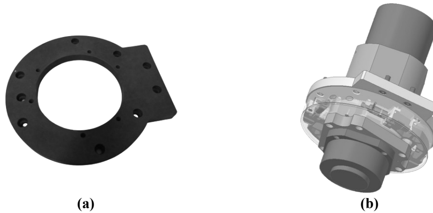
Figure 5. Device Connection to Spindle Housing: (a) Real Flange Adapter, (b) Simulated mounting
