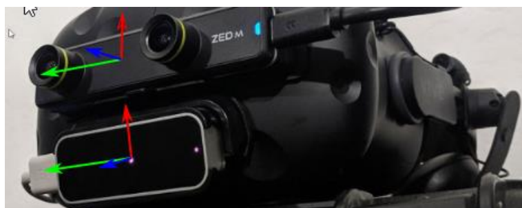
Figure 28: Zed Mini camera and LeapMotion position on the HTC Vive headset.
