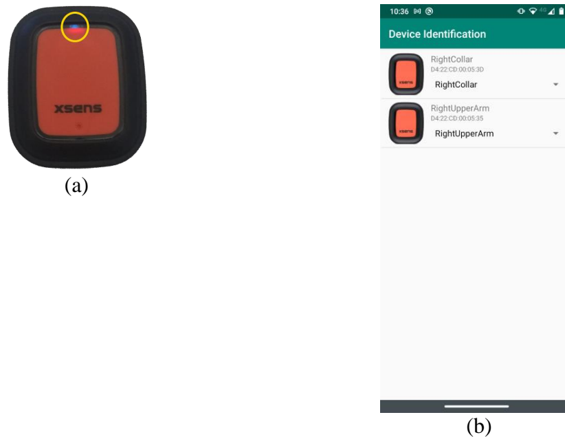
Figure 58: The XDot led position (a) and the XDot bone-to-device mapping page (b)
