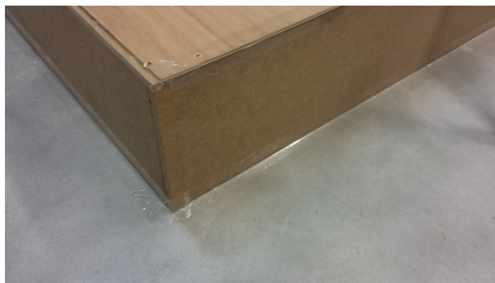
Figure 4: RRT sample box used as panel resonator; sealing detail
