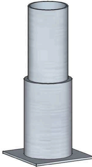
Figure 4: A 3D rendering of AB part, welded to the endplate and to the outer tube.
