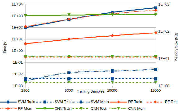
Fig. 4: Computational and memory footprint performance: training times— solid line , testing times— dashed line , and memory footprint— dotted line of the classifiers, versus the number of training samples
