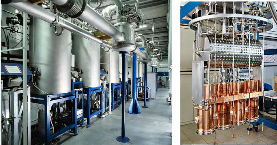
Figure 3.9: On the left: a section of the ALPI Linac with the cryostats containing superconducting cavities. On the right: the inside of a cryostat with 4 copper cavities.
